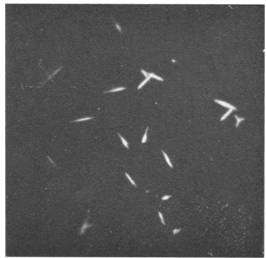
Figure 2 \text{Cu}^+ ion-analyser image of copper in (111) silicon slice. Primary \text{O}^+ beam ( \times 240 ).
